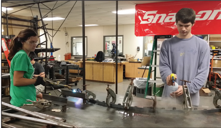
Mentor John Ivey helps Kayley Green-Tooney with the pit display. They are using an oxyacetylene torch to heat the bars for a bend curve to put in the acrylic display.
